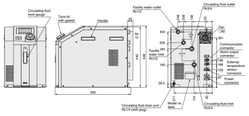
For NPT fitting specification (-N), all fittings (including those at the circulating fluid drain port) are made of NPT.
