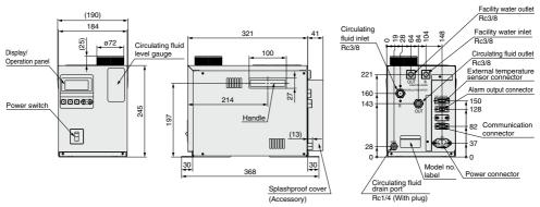
For NPT thread specification (-N), all fittings (including those at the circulating fluid drain port) are made of NPT.
