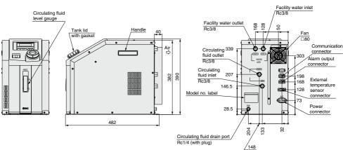
For NPT thread specification (-N), all fittings (including those at the circulating fluid drain port) are made of NPT.
